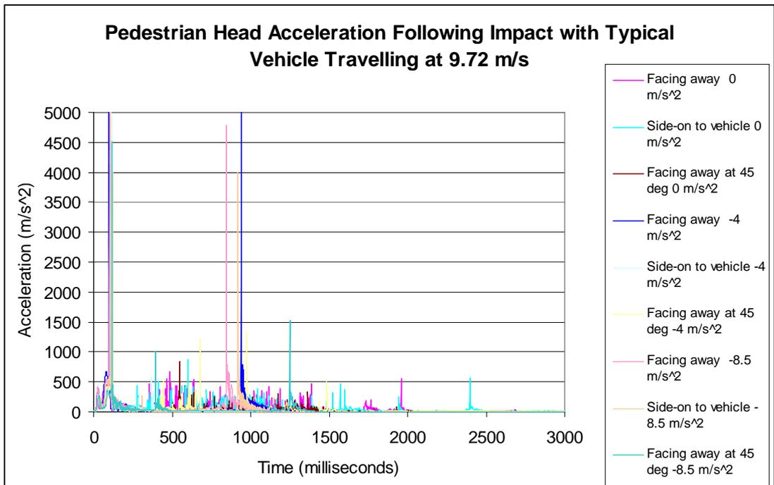
Figure 5.49 Head Acceleration for 5<sup>th</sup> Percentile Female MADYMO Human Model Struck by Typical Vehicle with the Vehicle Initially Travelling at 9.72 ms<sup>-1</sup>, Three Different Driver Actions (No Action, Moderate Braking and Heavy Braking) and Three Pedestrian Orientations (Facing Away from Vehicle, Side-On to Vehicle and Facing Away at 45°).
