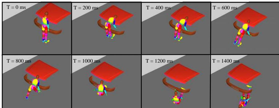
Figure 5.19 Pedestrian Motion Following Impact at  $4.4 \text{ ms}^{-1}$
