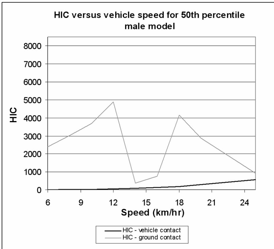
Figure 5.32. HIC Versus Vehicle Speed for 50<sup>th</sup> Percentile Male Model
