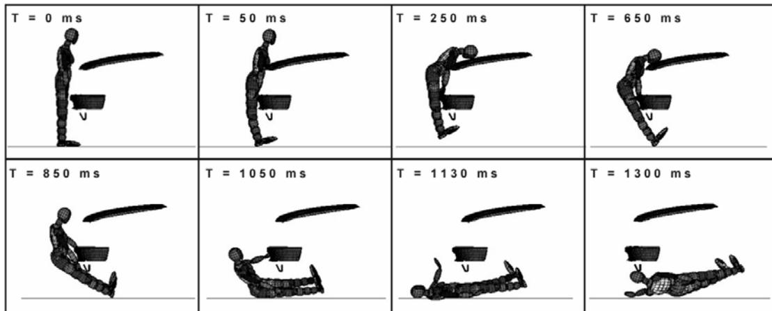
Figure 5.17. Impact Sequence at 2.8 ms<sup>-1</sup>
