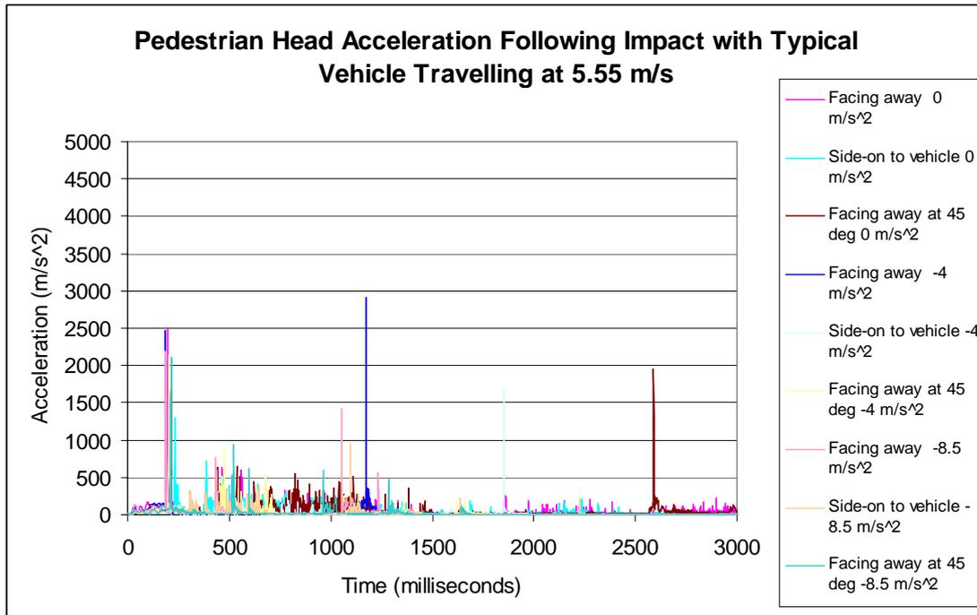
Figure 5.46 Head Acceleration for 5<sup>th</sup> Percentile Female MADYMO Human Model Struck by Typical Vehicle with the Vehicle Initially Travelling at 5.55 ms<sup>-1</sup>, Three Different Driver Actions (No Action, Moderate Braking and Heavy Braking) and Three Pedestrian Orientations (Facing Away from Vehicle, Side-On to Vehicle and Facing Away at 45°).
