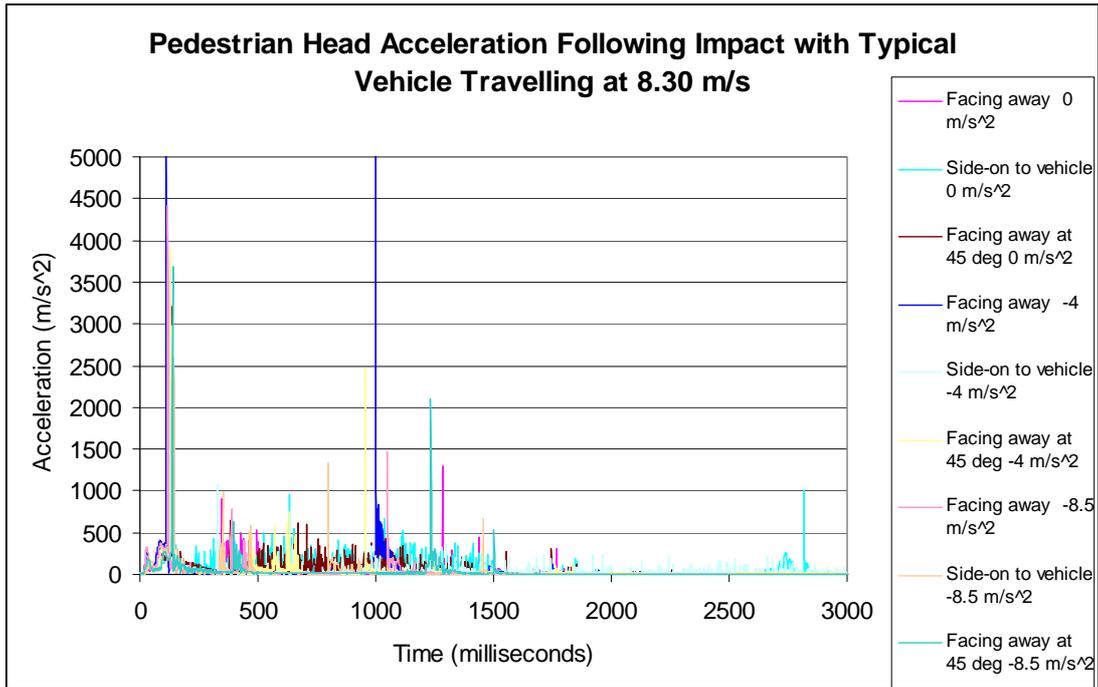
Figure 5.48 Head Acceleration for 5<sup>th</sup> Percentile Female MADYMO Human Model Struck by Typical Vehicle with the Vehicle Initially Travelling at 8.3 ms<sup>-1</sup>, Three Different Driver Actions (No Action, Moderate Braking and Heavy Braking) and Three Pedestrian Orientations (Facing Away from Vehicle, Side-On to Vehicle and Facing Away at 45°).
