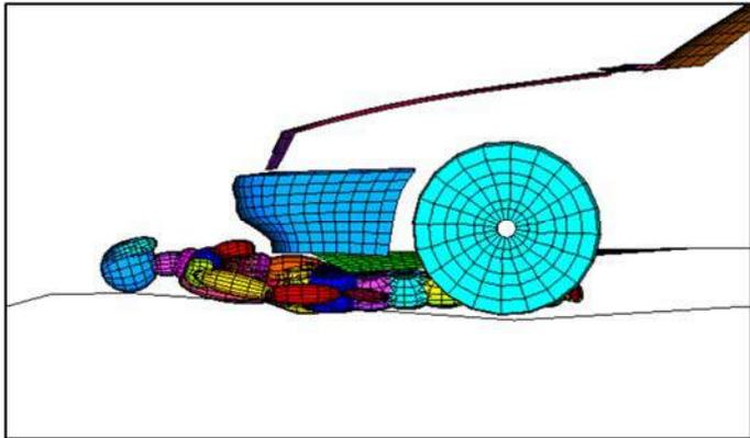
Figure 5.59: Vehicle Jammed Atop Pedestrian
