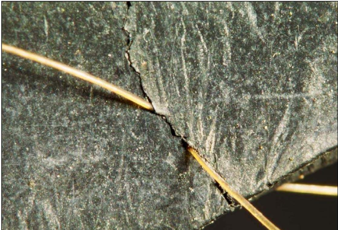
**Figure A(III).6 Hair from Pedestrian Trapped in Plastic at Base of Windscreen**
