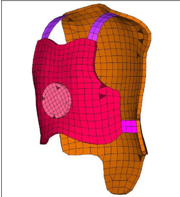
Figure A(I).10 Finite-Element Body Armour Model
