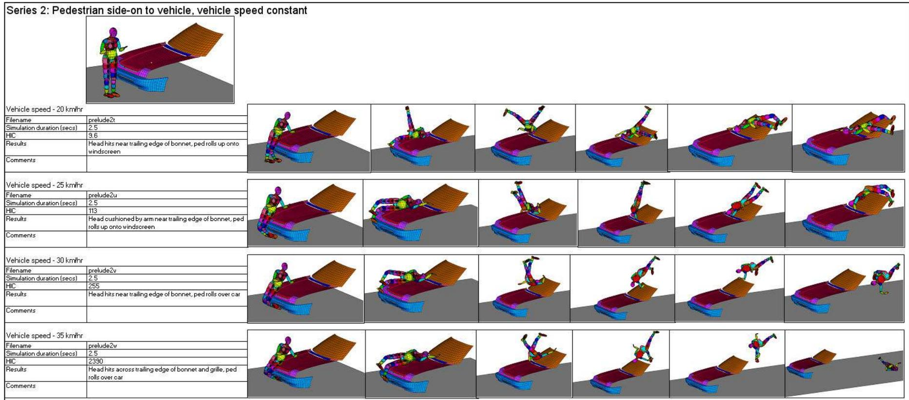
Figure A(III).12 Graphical Results From Series 2: Pedestrian Side on to Vehicle, Vehicle Speed Constant
