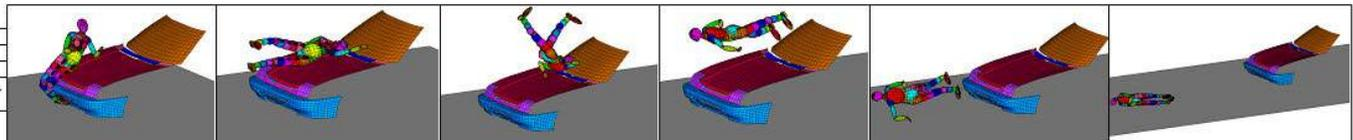
**Figure A(III).15 Graphical Results From Series 1: Pedestrian Side on to Vehicle, Vehicle Decelerating Heavily**
