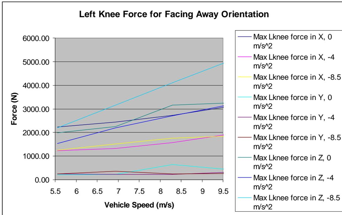
Figure 5.36 Left Knee Force for Facing Away Orientation
