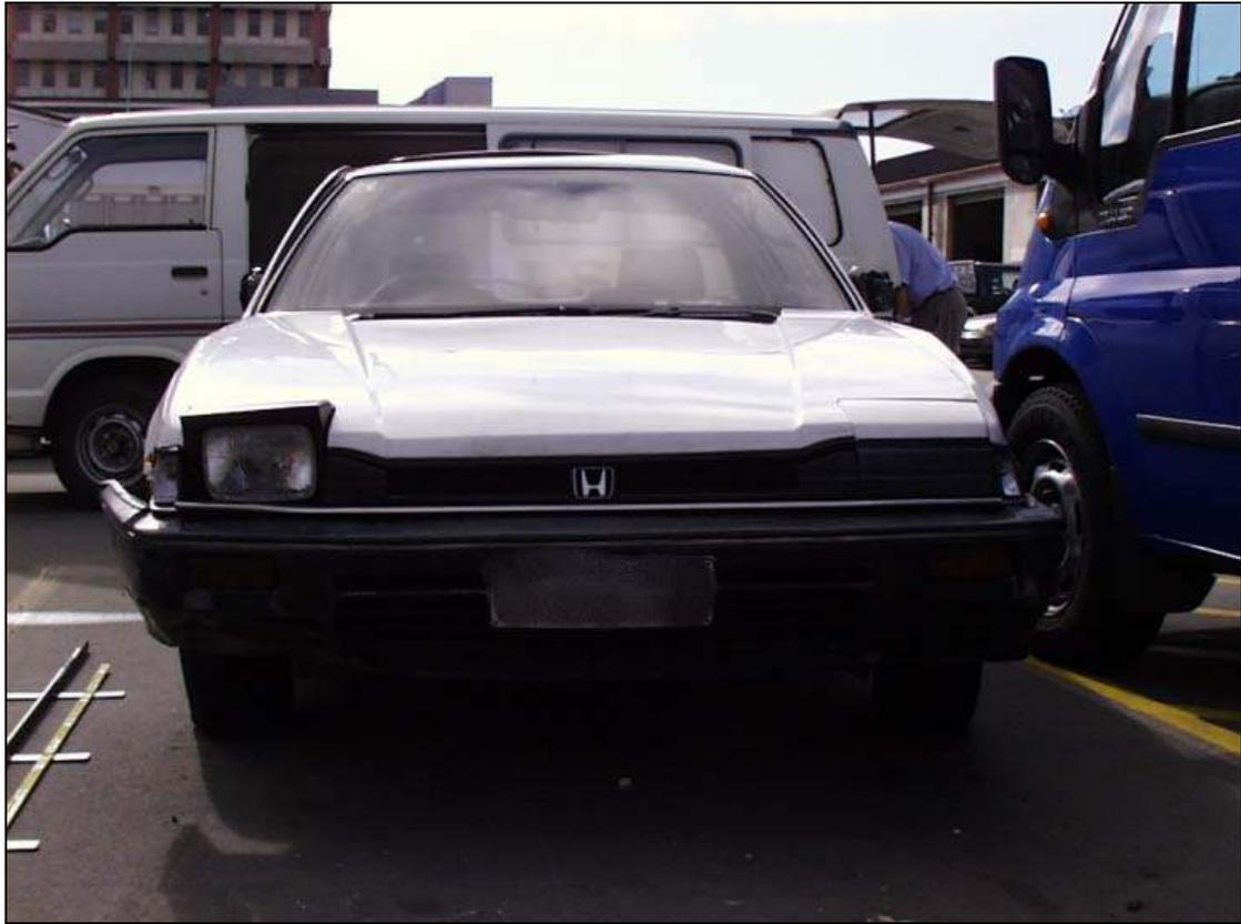
**Figure A(III).3 Front View of Vehicle Prior to Measurement – Note Rails for Coordinate Measuring System to Left of Vehicle. Headlight has been lifted for Inspection**
