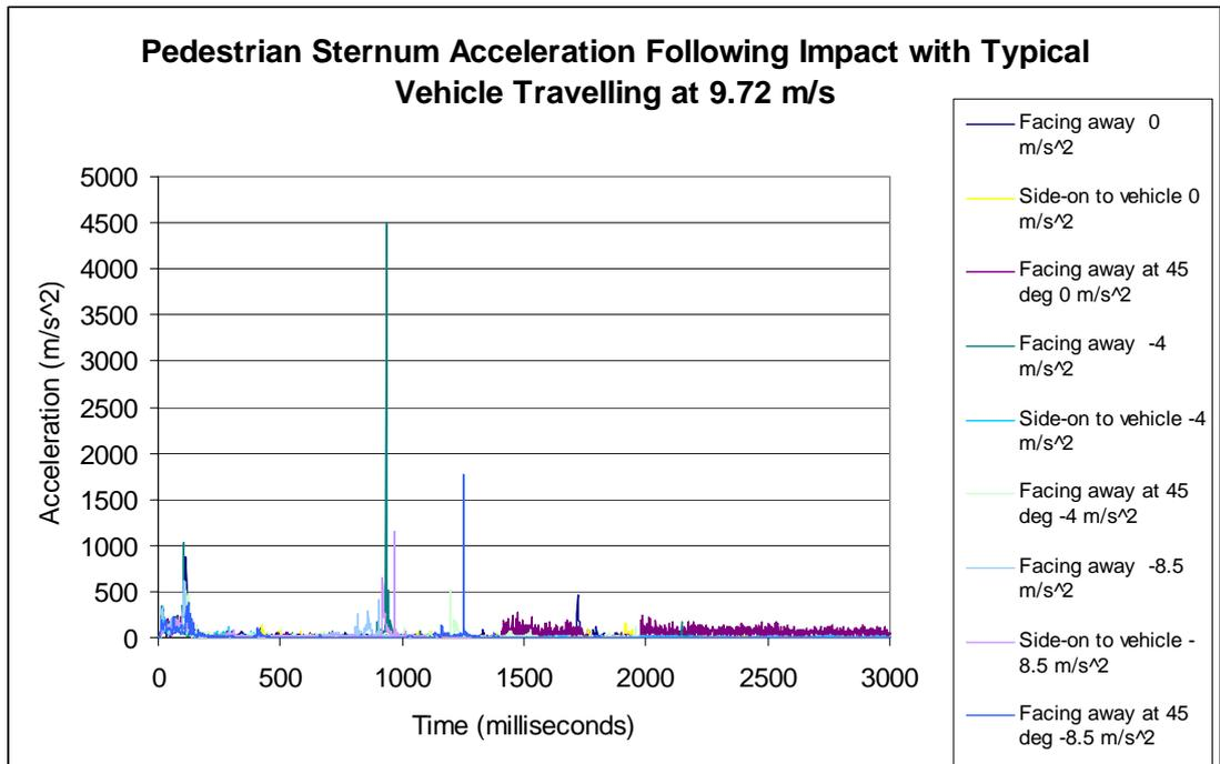
Figure 5.54 Sternum Acceleration for 5<sup>th</sup> Percentile Female MADYMO Human Model Struck by Typical Vehicle with the Vehicle Initially Travelling at 9.72 ms<sup>-1</sup>, Three Different Driver Actions (No Action, Moderate Braking and Heavy Braking) and Three Pedestrian Orientations (Facing Away from Vehicle, Side-On to Vehicle and Facing Away at 45°).
