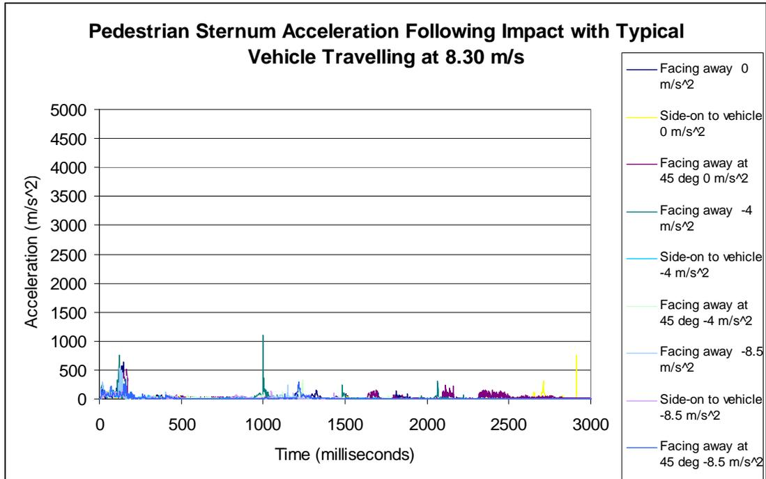
Figure 5.53 Sternum Acceleration for 5<sup>th</sup> Percentile Female MADYMO Human Model Struck by Typical Vehicle with the Vehicle Initially Travelling at 8.3 ms<sup>-1</sup>, Three Different Driver Actions (No Action, Moderate Braking and Heavy Braking) and Three Pedestrian Orientations (Facing Away from Vehicle, Side-On to Vehicle and Facing Away at 45°).
