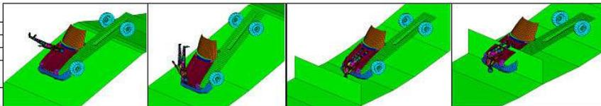
**Figure A(III).24 Graphical Results From Series 2: Pedestrian Lying on Back on Bonnet, Head Towards Windscreen**
