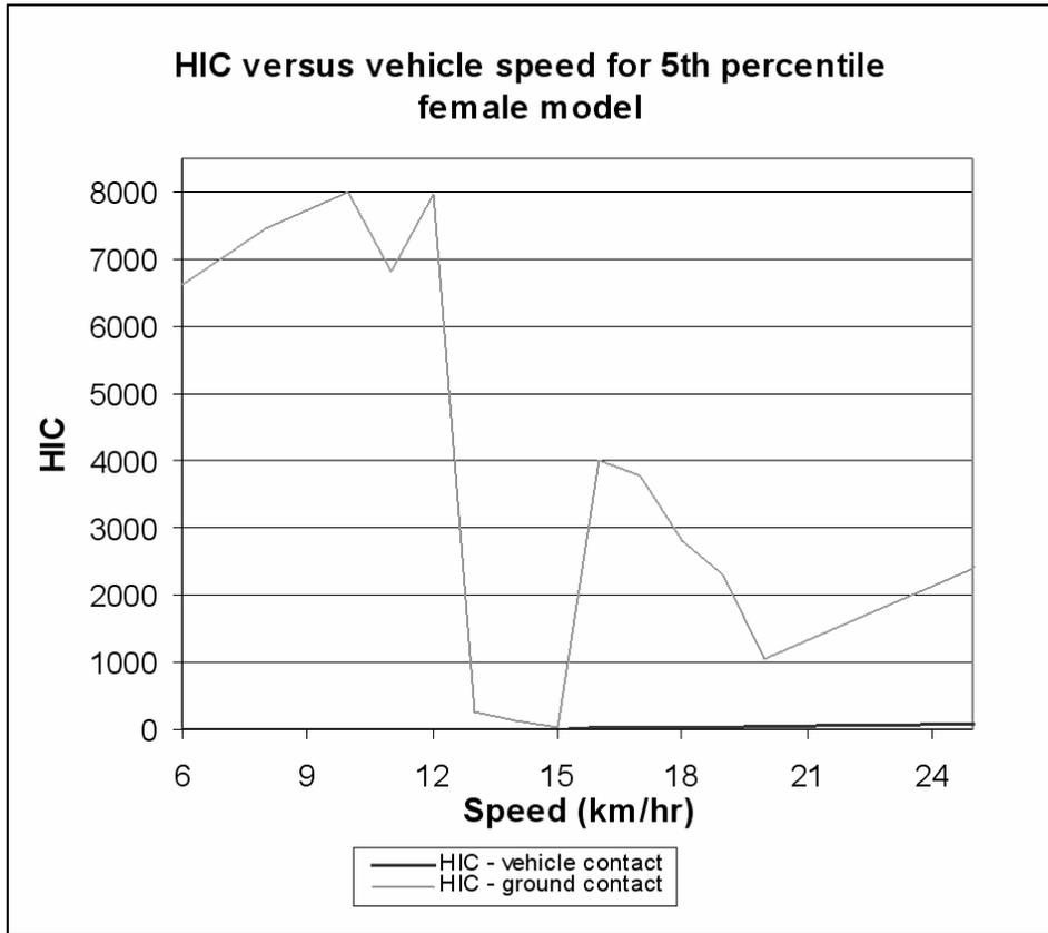
Figure 5.31: HIC Versus Vehicle Speed for 5<sup>th</sup> Percentile Female Model
