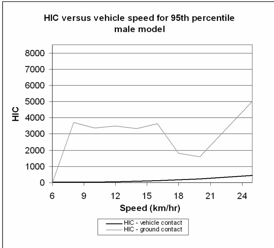
Figure 5.33. HIC Versus Vehicle Speed for 95<sup>th</sup> Percentile Male Model
