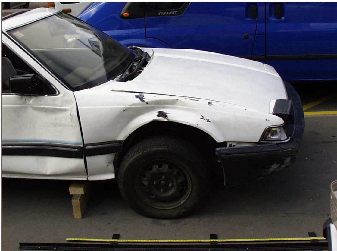
**Figure A(III).4 Side View of Vehicle Prior to Measurement – Note Rails for Coordinate Measuring System at Bottom of Photo. Damage to Vehicle Caused After and not related to Pedestrian Impact**
