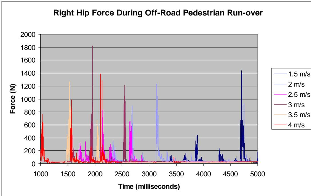
Figure 5.62: Right Hip Force during Off-Road Pedestrian Run-over
