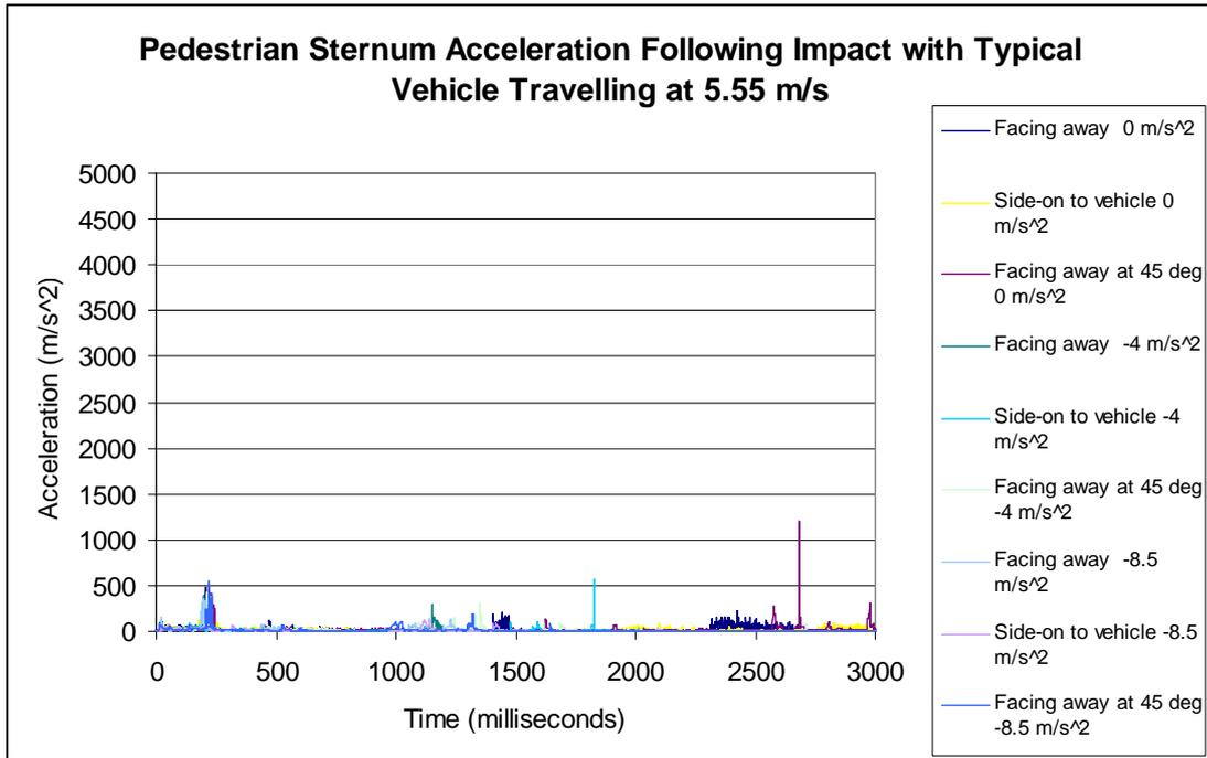
Figure 5.51 Sternum Acceleration for 5<sup>th</sup> Percentile Female MADYMO Human Model Struck by Typical Vehicle with the Vehicle Initially Travelling at  $5.55 \text{ ms}^{-1}$ , Three Different Driver Actions (No Action, Moderate Braking and Heavy Braking) and Three Pedestrian Orientations (Facing Away from Vehicle, Side-On to Vehicle and Facing Away at  $45^\circ$ ).
