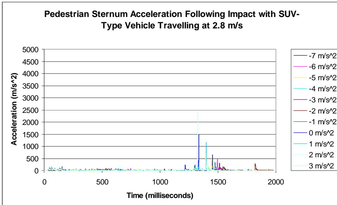
Figure 5.7 Sternum Acceleration for 5<sup>th</sup> Percentile Female MADYMO Human Model Struck by SUV-type Vehicle with the Vehicle Initially Travelling at 2.8 ms<sup>-1</sup>
