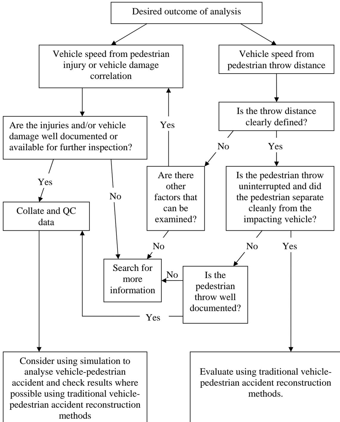
Figure 6.1 Flow-Diagram of Analysis Method versus Information Available
