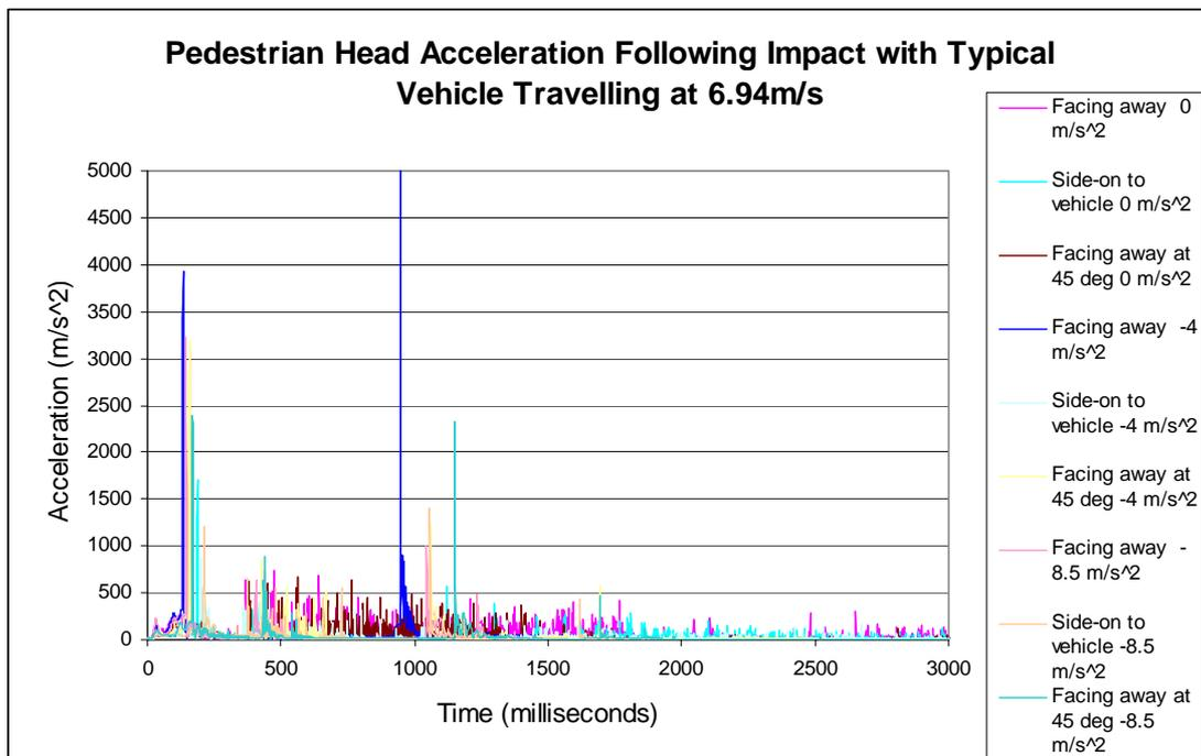
Figure 5.47 Head Acceleration for 5<sup>th</sup> Percentile Female MADYMO Human Model Struck by Typical Vehicle with the Vehicle Initially Travelling at 6.94 ms<sup>-1</sup>, Three Different Driver Actions (No Action, Moderate Braking and Heavy Braking) and Three Pedestrian Orientations (Facing Away from Vehicle, Side-On to Vehicle and Facing Away at 45°).
