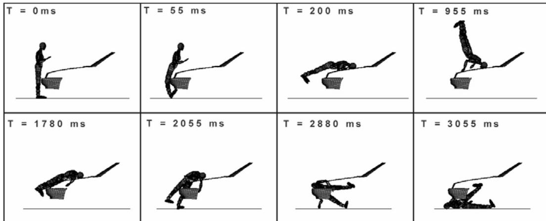
Figure 5.43. Impact Sequence at 16 km/h
