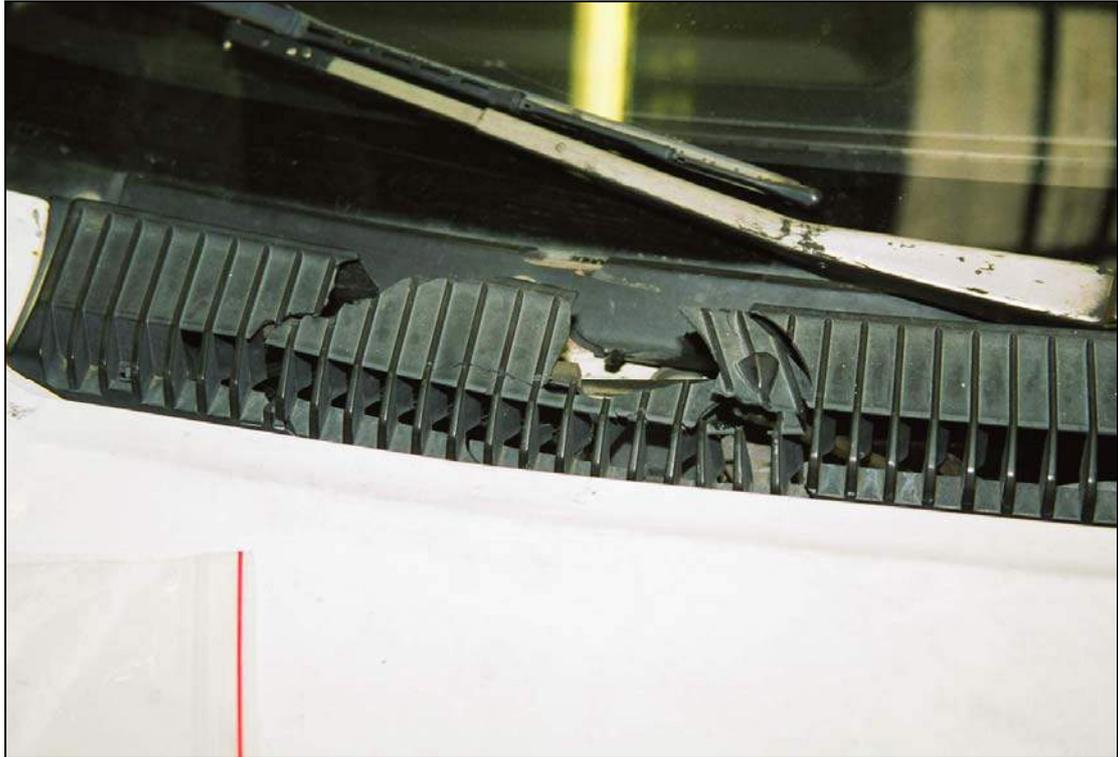
**Figure A(III).5 Damage to Grille at Base of Windscreen from Pedestrian Head Impact**
