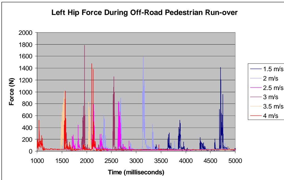
Figure 5.63: Left Hip Force during Off-Road Pedestrian Run-over
