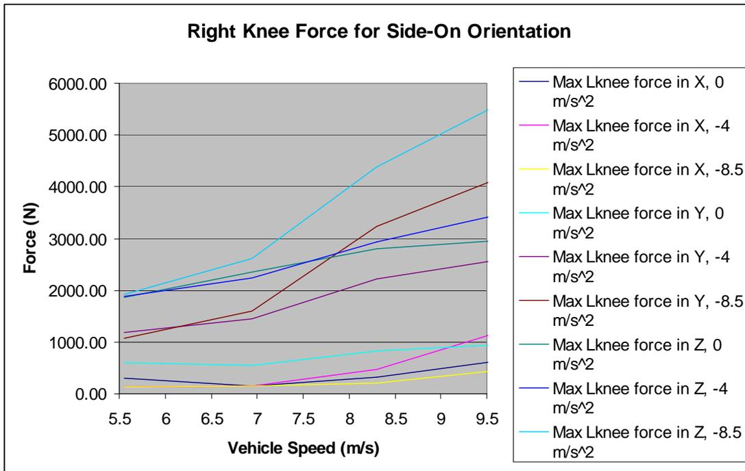
Figure 5.38 Right Knee Force for Side-On Orientation
