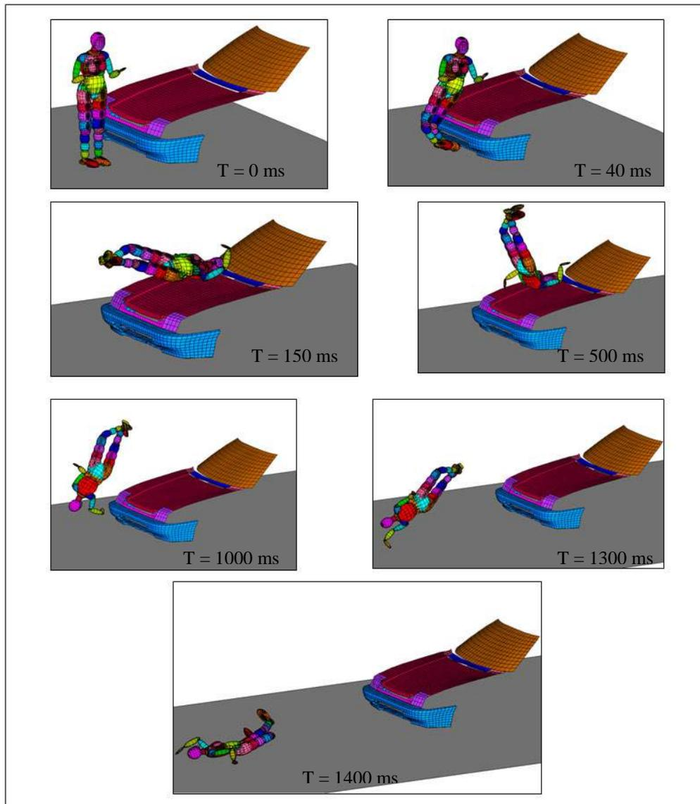
Figure 5.45: Vehicle Impact at 35 km/h, Vehicle Braking Heavily
