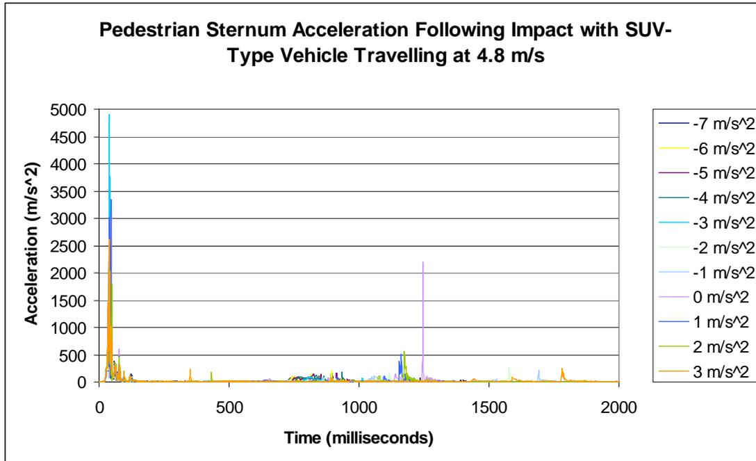
Figure 5.9 Sternum Acceleration for 5<sup>th</sup> Percentile Female MADYMO Human Model Struck by SUV-type Vehicle with the Vehicle Initially Travelling at 4.8 ms<sup>-1</sup>
