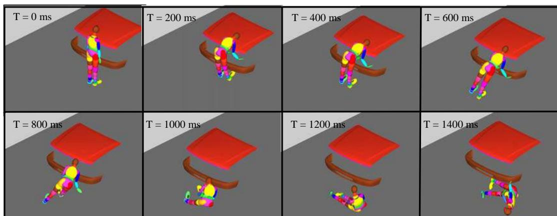
Figure 5.20 Pedestrian Motion Following Impact at  $4.8 \text{ ms}^{-1}$
