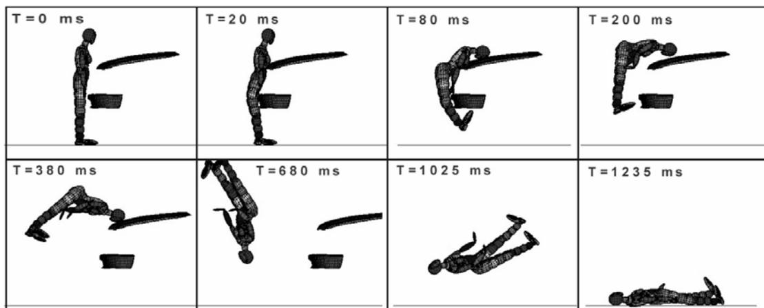
Figure 5.18. Impact Sequence at 6.9 ms<sup>-1</sup>
