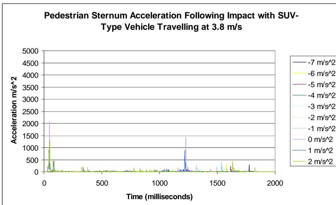
Figure 5.8 Sternum Acceleration for 5<sup>th</sup> Percentile Female MADYMO Human Model Struck by SUV-type Vehicle with the Vehicle Initially Travelling at 3.8 ms<sup>-1</sup>
