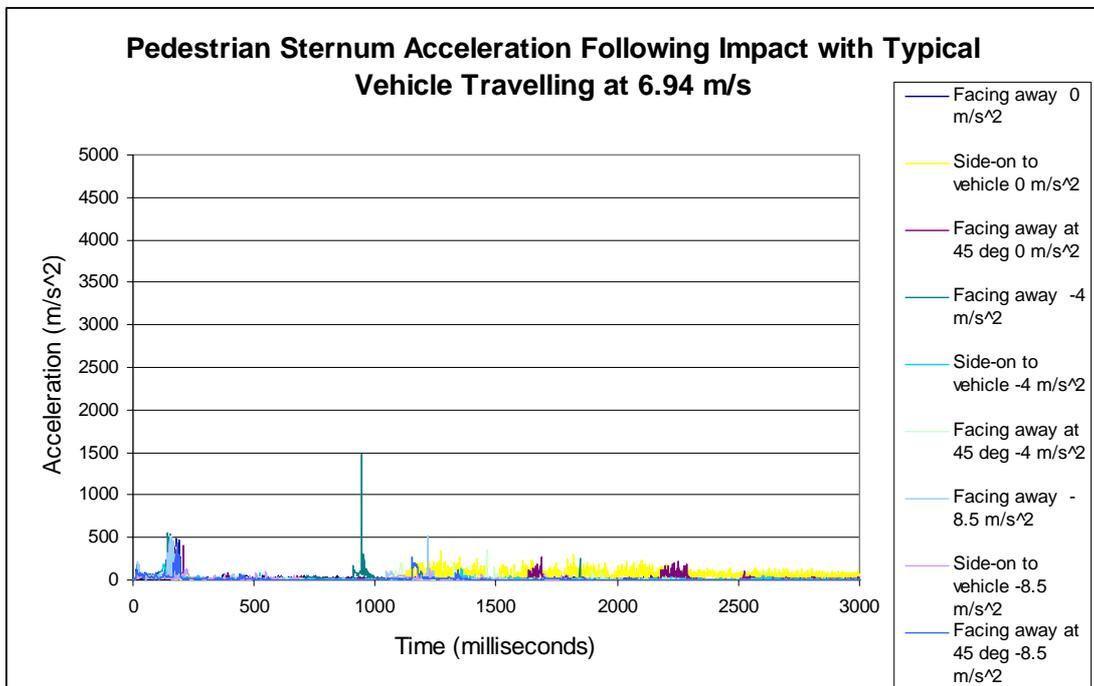
Figure 5.52 Sternum Acceleration for 5<sup>th</sup> Percentile Female MADYMO Human Model Struck by Typical Vehicle with the Vehicle Initially Travelling at  $6.94 \text{ ms}^{-1}$ , Three Different Driver Actions (No Action, Moderate Braking and Heavy Braking) and Three Pedestrian Orientations (Facing Away from Vehicle, Side-On to Vehicle and Facing Away at  $45^\circ$ ).
